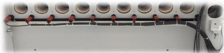
The temperatures are separately controlled on each heating element, and between the upper and lower side of rollers, by means of special thermocouples and related self-regulators. Each heating element is fitted with a hot air forced convection system in a closed circuit for maximum energy saving, composed of one ventilator controlled by inverter, and a battery of special diffusers.
