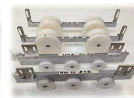
(roller change pitch device to manage different pitch and different rollers diameter )
